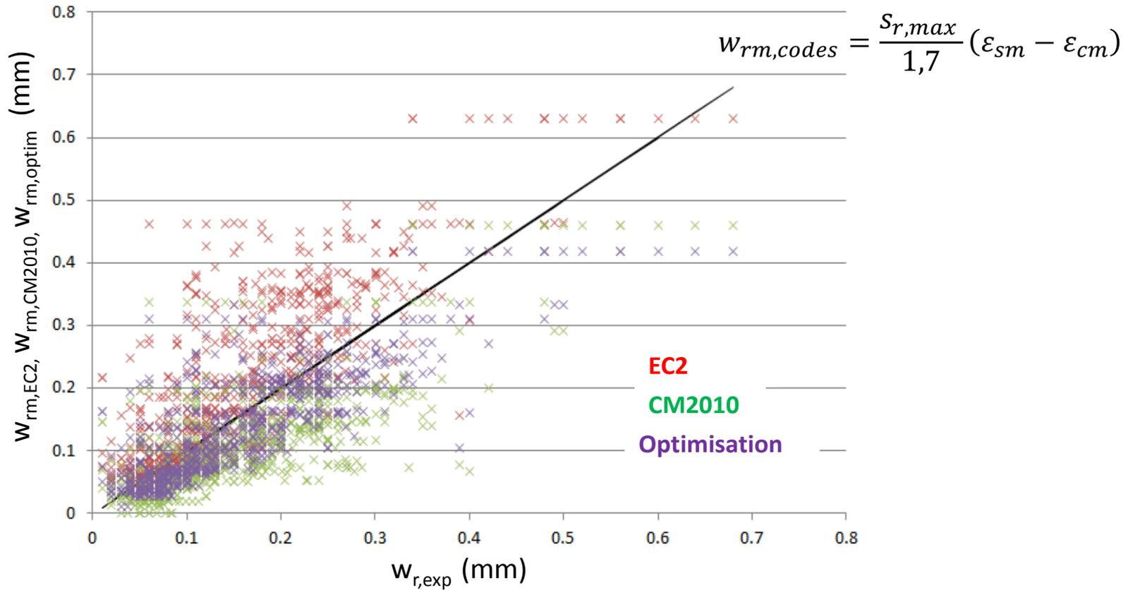
$$W_{rm, optim} = S_{rm} \frac{\sigma_s - 0,6 k_t \frac{f_{ctm}}{\rho} (1 + \alpha_e \rho)}{E_s} \quad \text{with } S_{rm} = 1,37c + 0,117 \left( \frac{\phi}{\rho} \right)$$
